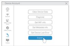
This tool is also helpful in checking setup failure reasons, MAC address, and offline charts. You can also use it to export offline data stored in the device internal memory.
